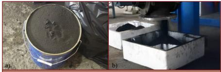
Dry residue: a) dry subsoil (from oil sludge processing), b) carbon black (from waste rubber products processing)
